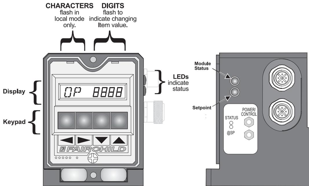
**Figure 2. Model T1750 Series Transducer Keypad Functions**
